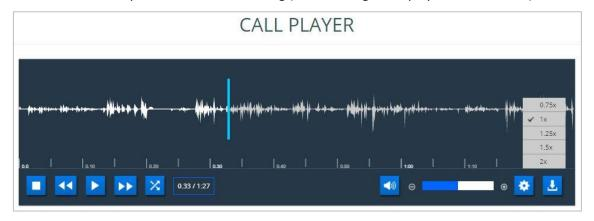
The cog enables the speed of the call recording playback to be selected and the download icon triggers a download of the call recording as a .wav file.
